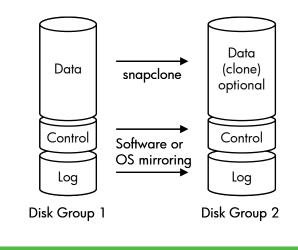
If disk group 2 does not contain the snapclone of the data files, the number of disks in disk group 2 should be determined by the sequential performance demand of the log workload. Typically, this results in more usable capacity than is required for the logs. In this case, choose Vraid1 for the log disks. Vraid1 offers the highest availability and, in this case, does not affect the cost of the solution.
